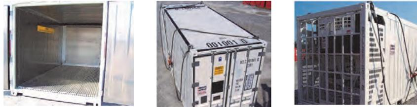
Mesh doors guard around the generator and refrigeration unit providing access for maintenance with protection and ventilation for the equipment.
